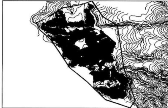
Figure 1. Graphical display of optimal mix of skidding methods. Darker areas represent areas where ground skidding is preferable and lighter areas represent where aerial methods are preferred. Thick lines indicate areas where roads should be constructed. Dark spots within lighter areas indicate tower location.
